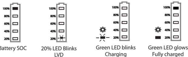
In Normal Operation, the controller shows the state of Charge of the battery and the solar panel activity.
