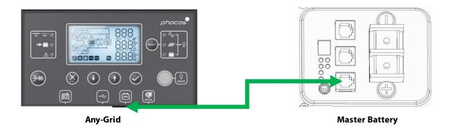
5. Ensure the battery modules are wired as outlined in the Arco battery manual. Turn on the batteries:
