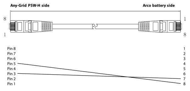
• Battery communication cable with **only** the following pins connected:
