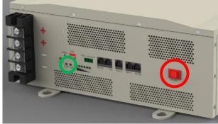
6. Turn the "ON/OFF" load power button of the Any-Grid(s) to the ON position (depressed), but make sure no loads are connected:
