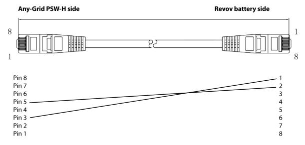
Make sure the cable is correctly oriented between the battery and PSW-H unit when installing below.
