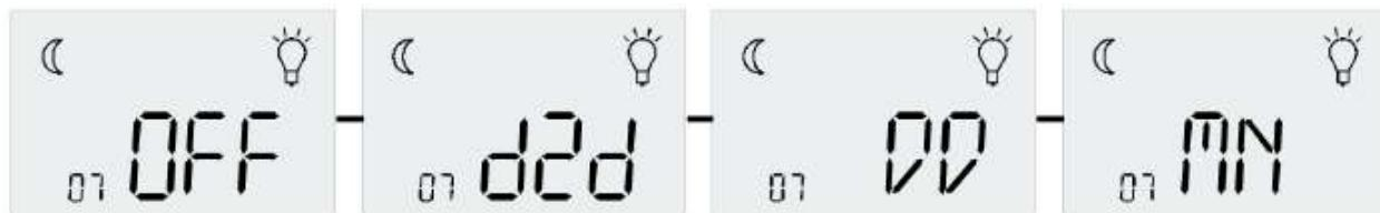
When the LCD shows the DD setting, press SET to save the setting. The DD setting will flash briefly to confirm the selection.
