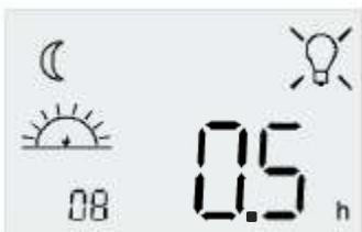
When the LCD shows the 0.5 setting, press SET to save the setting. The 0.5 setting will flash briefly to confirm the selection.
