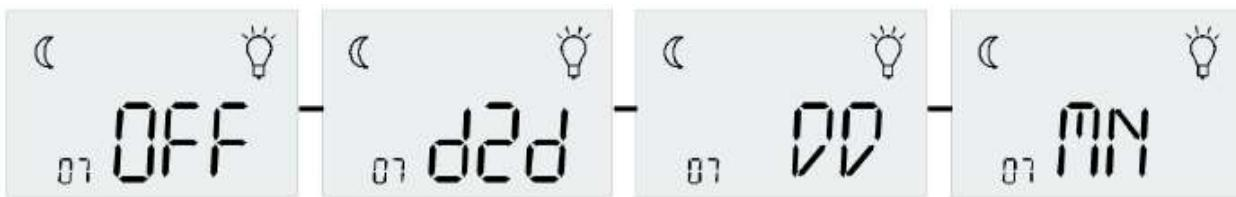
When the LCD shows the D2D setting, press SET to save the setting. The D2D setting will flash briefly to confirm the selection.
