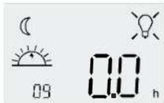
When the LCD shows the 0.0 setting, press SET to save the setting. The 0.0 setting will flash briefly to confirm the selection.
