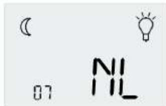
Use the UP or DOWN arrow key to navigate the nightlight submenu. The previously selected setting will flash.
