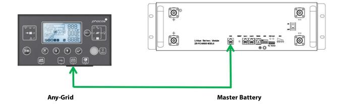
5. Ensure the battery modules are wired as outlined in the ZRGP battery manual. Turn on the batteries with their ON/OFF switch:
